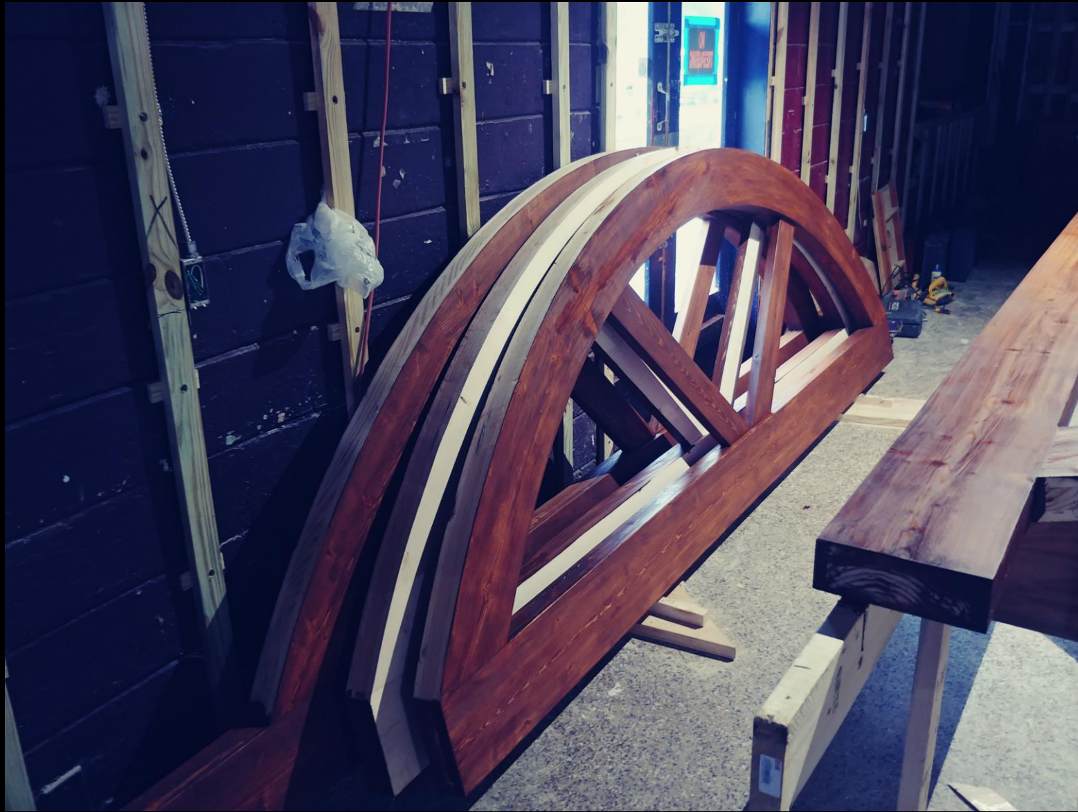
Arched Beam Trusses ready for Installation
